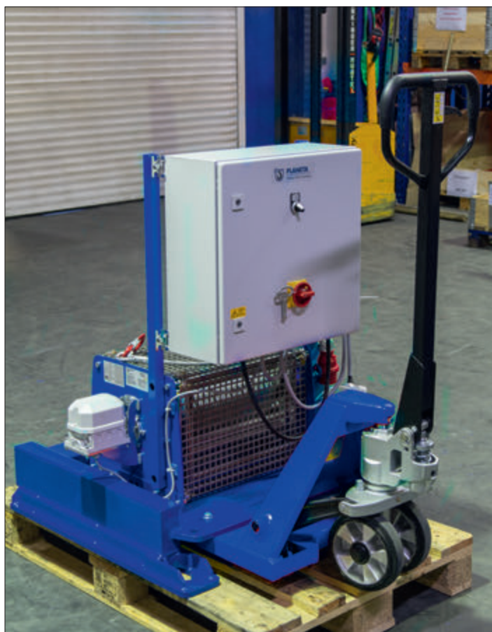
PFW-E 3000 as a mobile pulling winch for railway maintenance
