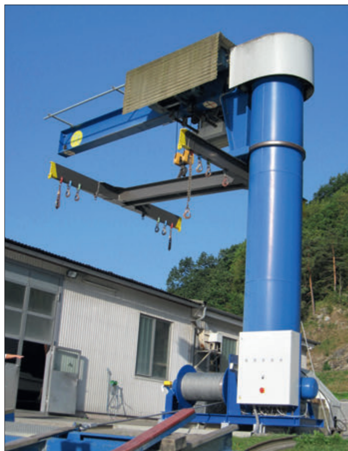
SB-E 309 as a slipway winch for sports boats
