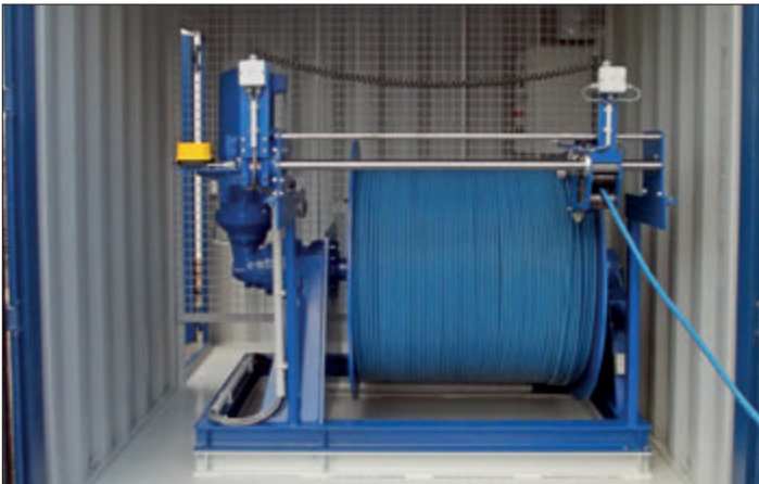
SB-E 306 as a surveying winch with 1,800 m data cable
