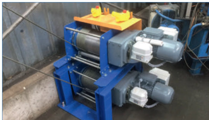
PFW-E 1000 as a double winch block for a test bench
