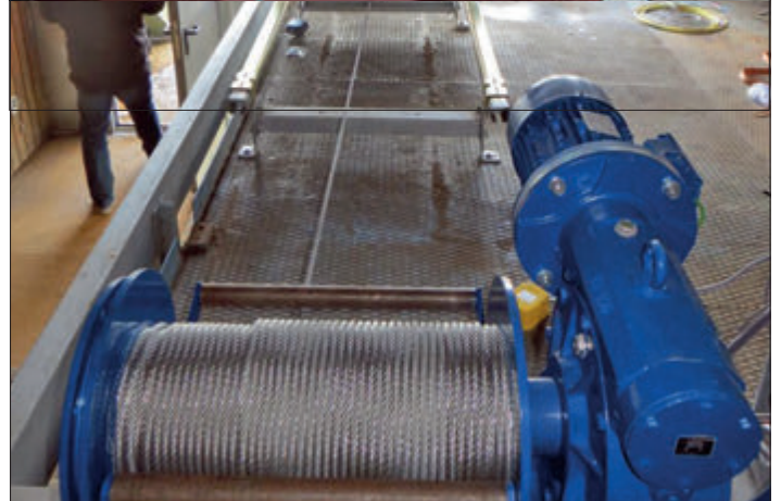
MC-E 2200 as a hoist winch for lane milling on ski jumps
