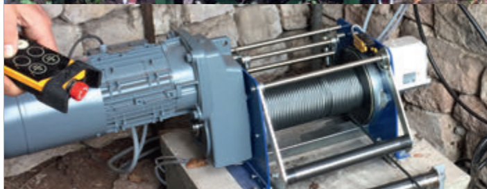
PFW-E 1000 as the drive of an inclined elevator
