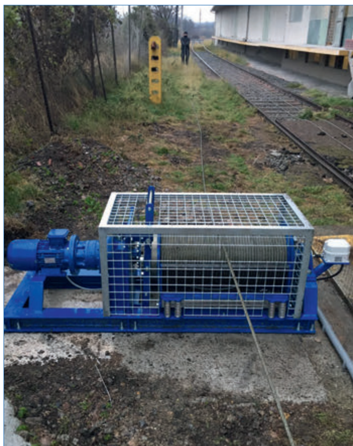
PHW-E 305 as a traversing winch on a wagon filling station
